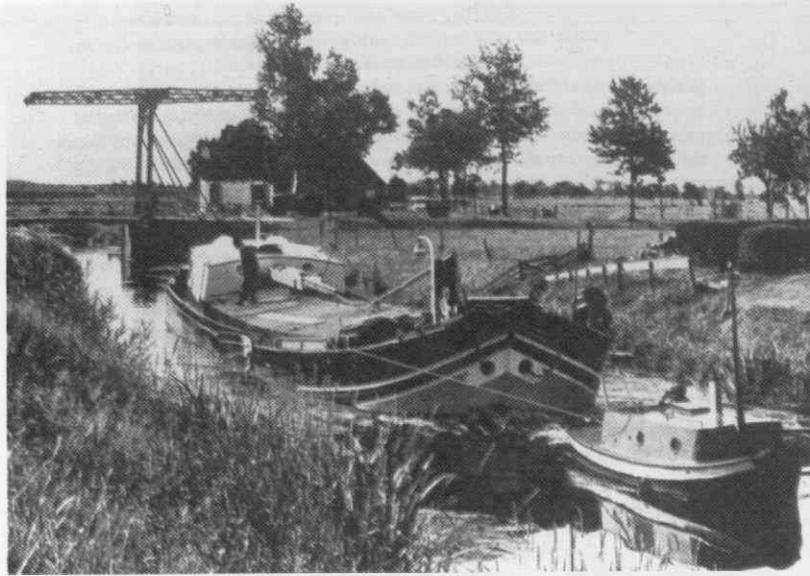
9. The use of engines did replace the hand- and wind power. In the beginning they were searching for a solution, for example with a tug boat. Here we see an iron sailing barge in a small canal in the north of Holland who got rid off his mast and sails, and used a special made tugboat for sailing.
